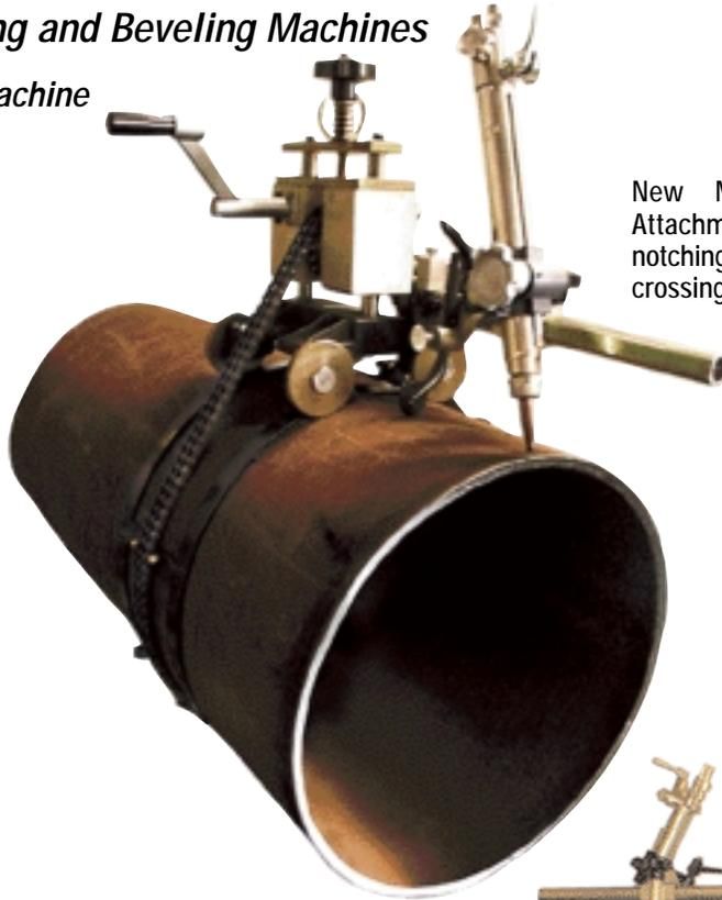
New Mini Out-of-Round Attachment minimizes the notching of the pipe when crossing weld seam.
